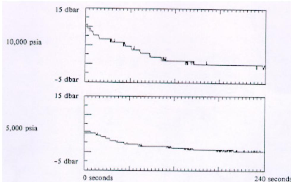
During calibration, the sensors are allowed to *warm-up* before calibration points are recorded. Similarly, for best depth accuracy the user should allow the CTD to *warm-up* for about 2 minutes before beginning a profile; this can be part of the *soak* time in the surface water. *Soaking* also allows the CTD housing to approach thermal equilibrium (minimizing the housing's effect on measured temperature and conductivity) and permits a Beckman- or YSI-type dissolved oxygen sensor (if present) to
