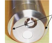
Wrench flats on end cap. Note: If your 39-IM has an external thermistor, remove temperature guard to access wrench flats
