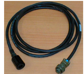
Deck Unit to 9plus test cable
