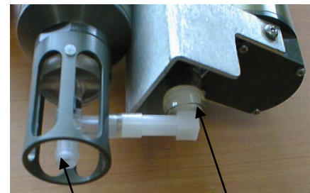
Do not remove TC Duct for rinsing, cleaning, or storage – attach Tygon tubing to end of TC Duct to loop Tygon tubing to each end of cell
