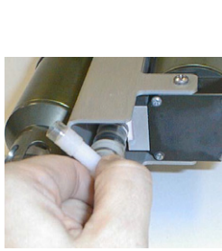
Rotate C Duct clockwise
