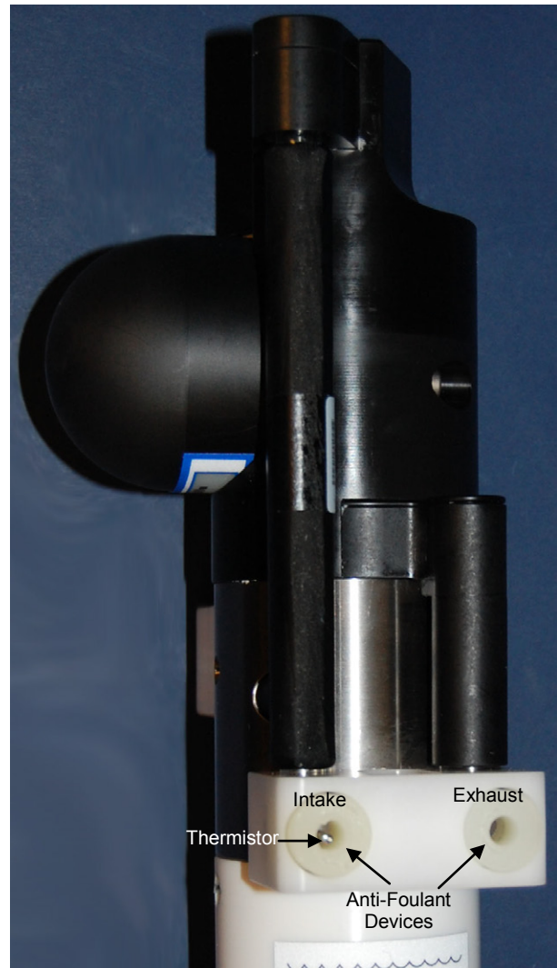
Shown with conductivity cell guard removed
