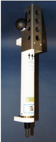
Plastic ShallowCAT housing shown; titanium housing available
