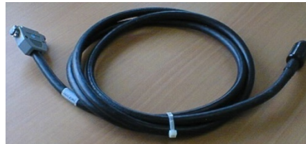
Serial Test Cable – connects SBE 44 to computer to test serial communications through SBE 44's RS-232 bulkhead connector
