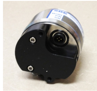
SBE 63 (titanium housing)
