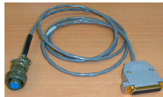
Navigation Interface test cable (Interface Box to NMEA navigation device simulation computer)
