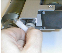
Rotate C Duct clockwise
