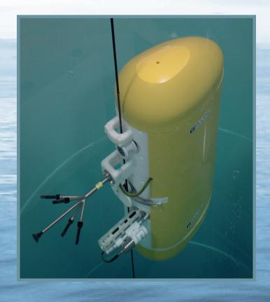
McLane Moored Profiler (MMP) shown with integrated Sea-Bird 52MP CTD and inductive modem telemetry
