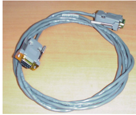
171887 Computer to Deck Unit cable for Serial Data & Carousel Data connectors (2 cables / SBE 33)
