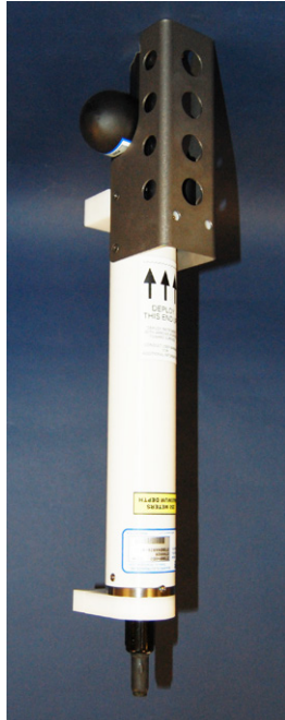
SBE 37-SMP-ODO (AF24173 Anti-Foulant Devices installed at Sea-Bird)
