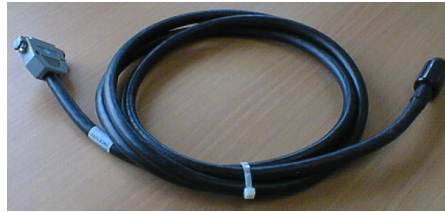
801434 test cable – connects SBE 44 to computer to test serial communication through SBE 44's RS-232 bulkhead connector
