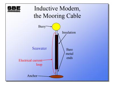
The second current loop is made by the mooring cable itself and seawater. The cable is bare metal on the top and bottom and insulated in the middle.
