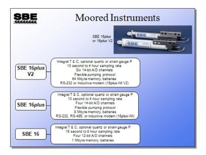
The SBE 16, 16*plus*, and 16*plus* V2 are moored versions of the SBE 19 family of SeaCATs. The 16*plus* V2 is actually a 19*plus* V2 in moored mode, with optional pressure sensor. These instruments have the capability to power external sensors and log analog A/D data from them. This is the instrument of choice if you require more data than C, T, and P.
