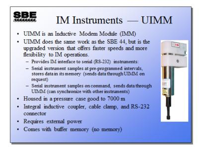
The UIMM provides more flexibility in programming than the SBE 44, allowing for connection to a wider number of RS-232 instruments. Unlike the SBE 44, the UIMM requires external power.
