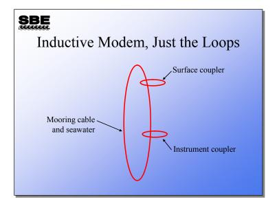
Here is a very simple view of the communication links. Note that there can be up to 100 instrument couplers on the mooring cable – seawater loop.
