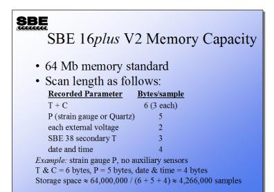
The SBE 16*plus* V2 has considerably more memory than the 16 or 16*plus*, with 64 Mbytes of non-volatile flash memory. Again, memory capacity depends on the configuration of the instrument.
