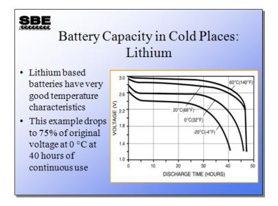
Lithium batteries offer better performance. The main drawback to using them is international shipping restrictions on lithium. For example, looking at the lithium batteries for the SBE 37 MicroCATs and SBE 44 Underwater Inductive Modem:
