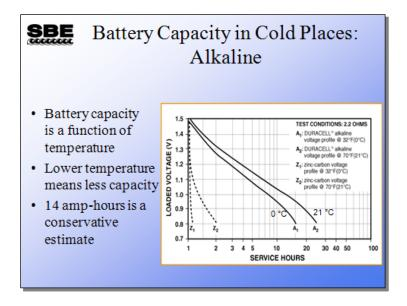
Considering the time and money involved in making a mooring, fresh batteries are a small expense. We estimate the battery life in an SBE 16, 16*plus*, or 16*plus* V2 assuming that it begins with 14 amp-hours of power. As you see from the plot, 14 amp-hours is a conservative estimate. At 0 °C an alkaline battery is expected to supply 0.8 volts after 15 hours of continuous service (i.e., continuous sampling, not the intermittent sampling usually done with moored instruments).
