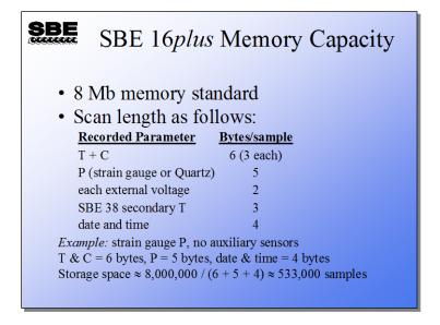
The SBE 16*plus* has considerably more memory than the 16, with 8 Mbytes of non-volatile flash memory. Again, memory capacity depends on the configuration of the instrument.
