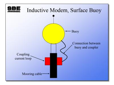
The first current loop is made around the mooring cable. The coupler is a ferrite donut. Ferrite is the stuff that magnetic tape is made from. The electrical current that flows around the coupler induces a current that flows through the mooring cable and the seawater. Thus, the modem signal is transmitted by the surface buoy into its coupler, and the coupler induces a current in the seawater and mooring cable.
