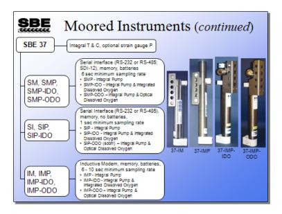
Like the SBE 16 SeaCAT family, the SBE 37 MicroCATs have integral T and C sensors, and may also be equipped with a pressure sensor. It comes in three main types:
