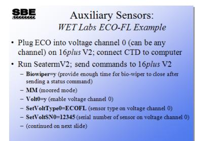
As mentioned earlier, when enabling/disabling a parameter, y and 1 are equivalent, and n and 0 are equivalent (i.e., **Volt0=y** and **Volt0=1** both enable voltage channel 0). The commands for enabling/disabling each voltage channel are **Volt0=** through **Volt5=**.
