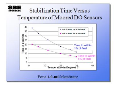
**Prior to 2007, all SBE 43s were sold with a 0.5-mil thick membrane.** Beginning in 2007, Sea-Bird began offering two membrane thicknesses – 0.5 mil (faster response, typically for profiling applications and 1.0 mil (slower response but more durable, typically for moored applications). This plot is for a **1.0-mil membrane**.
