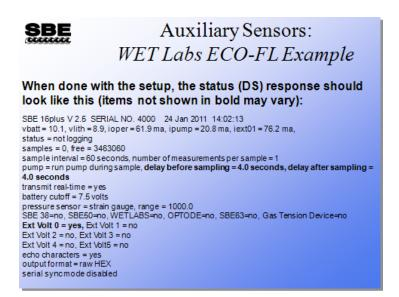
When the setup is complete, the **DS** response should show the values you entered for delay before sampling and delay after sampling, and **Ext Volt0 = yes** (you enabled voltage channel 0, so the CTD will supply power to that channel and incorporate data from that channel into the CTD data stream). Additionally, because we set **Biowiper=y**, the response shows wait 4 seconds for biowiper to close
