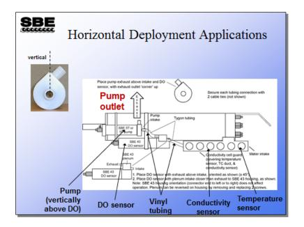
Notice here that the pump exhaust is now the highest point on the plumbing.
