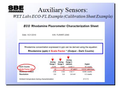
Here is an example calibration sheet from WET Labs. This calibration sheet is for an ECO-FL set that measures Rhodamine; it shows the Dark Counts and Scale Factor to input in the Sea-Bird configuration file.
