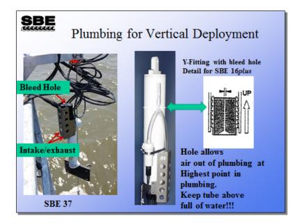
On the right, SBE 16*plus* TC intake is lowest on package, so it is the first thing to see the water in the plumbing.
