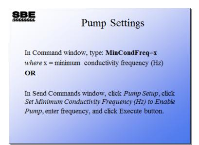
Set the Minimum Conductivity Frequency for the pump turn on signal. To prevent pumps from running dry, the pump will turn on only after a minimum conductivity value is measured by the conductivity sensor (an indication the instrument is in the water). You can control this by setting the frequency for the type of water you are working in.
