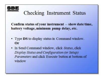
The status report contains much valuable information that allows you to confirm the instrument setup before deployment.
