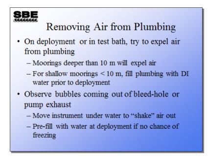
If you do not see air bubbles coming out of the bleed hole, the hole maybe clogged. Use a fine gauge wire to clear the bleed hole.
