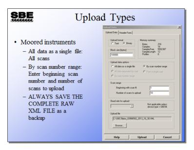
**Upload Format**: Seaterm232, Seaterm485, and SeatermUSB can upload in text or binary. Binary is approximately twice as fast; the resulting output file is the same, regardless of which upload method you use.
