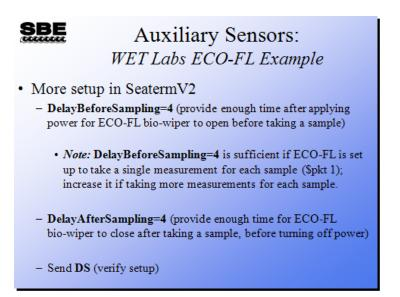
The CTD samples at user-programmable intervals for moored applications. It turns off power to the CTD and auxiliary sensors between measurements, conserving battery power. If integrating with a sensor with a bio-wiper, these settings are important:
