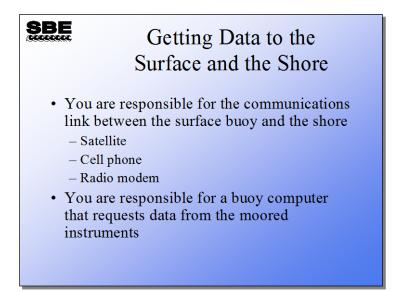
The complete inductive mooring system requires a computer at the surface, to send commands to the instruments via the surface inductive modem and to communicate with the shore. Sea-Bird has customers that use satellites, some that use cell phones, and some that use radio modems. It is your responsibility to develop the hardware and software to perform these duties.
