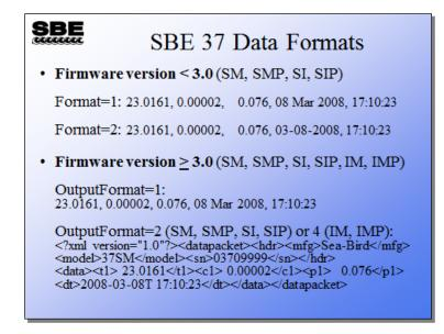
The basic data format is temperature, conductivity, pressure (if installed), date and time.
