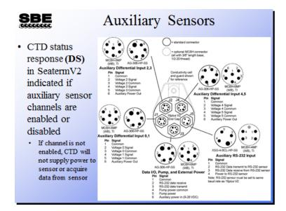
Sea-Bird CTDs can be configured with a wide range of auxiliary sensors. For example, the SBE 16*plus* V2 has three 6-pin bulkhead connectors for voltage output (0-5 volt) auxiliary sensors, each of which can accommodate two sensors (using a Y-cable). It also has one 4-pin bulkhead connector for an RS-232 output sensor. The connectors provide power to and acquire data from the auxiliary sensors.
