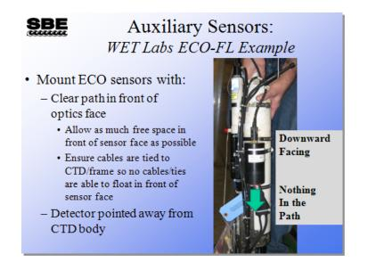
Attach the ECO on the CTD-cage or to the CTD. Preferred orientation is optical window facing down, to prevent sediment from settling on the window and to prevent sunlight from above from affecting the measurement. Be sure nothing is in the direct path of the optical window, and that nothing can reflect light back towards the sensor.
