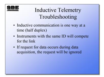
The inductive link is half duplex. This means that only one device on the link may be actively transmitting data at a time. If the situation occurs where two devices are trying to transmit, the communication will be corrupt.
