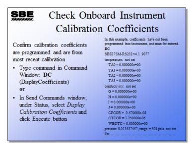
The calibration coefficients programmed into the instrument are used if outputting data in engineering units through a terminal program. Verify the coefficients are correct, and match the most recent calibration sheets that you received from Sea-Bird.
