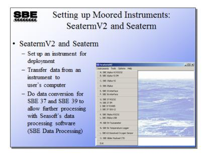
Even in moorings that use inductive telemetry, the data that is stored in the instrument is of interest. There may be occasions where the link between the surface buoy and the ground station malfunctioned, or the telemetered data may be a subset of that collected by the remote instrument. SeatermV2 and Seaterm provide the facility for data transfer and for the conversion of SBE 37 and SBE 39/39*plus* data to a format that can be used by the processing programs in Seasoft.
