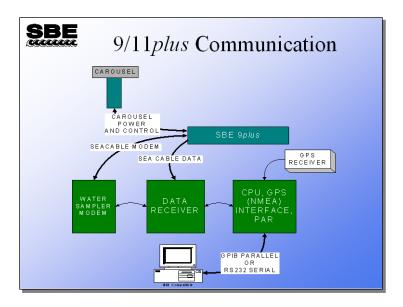
Here is a signal flow diagram for the circuit boards in the 11*plus*, the 9*plus*, the Carousel, and your PC. Note that water sampler commands pass from your computer to the 11*plus* CPU board, to the receiver board, to the modem board, to the 9*plus*, and into the Carousel.
