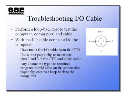
If the I/O cable fails this test, disassemble the hood part of the cable connector at the computer end of the cable, and check the solder connections.
