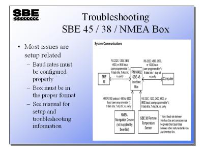
Sea-Bird manufactures an interface box specifically for the use with SBE 45 MicroTSG thermosalinograph, called the *SBE 45 Power, Navigation, and Remote Temperature Interface Box*. Note that the **baud rate between the Interface Box and the computer must be greater than the baud rates between the other instruments / devices and the Interface Box**.
