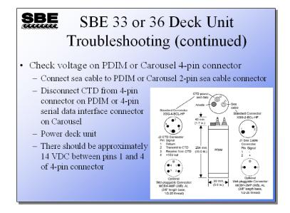
This test is useful for checking if power is going to the CTD.
