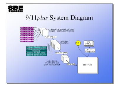
The 9/11*plus* is a highly modular system. You can exploit this characteristic of the instrument in troubleshooting. You can swap sensors, swap cables, and if necessary, swap printed circuit boards to see if trouble follows any one of these components.
