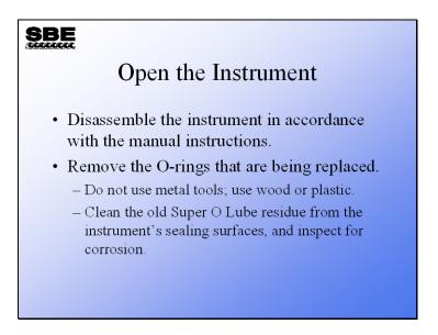
Make sure the instrument is completely dry before opening. Water on the electronic circuits can severely damage the instrument.
