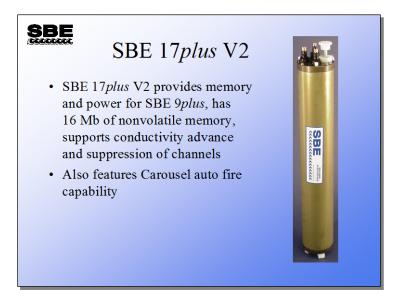
The SBE 17*plus* V2 acts as battery power and internally recording memory for the SBE 9*plus*. This device has the capability to close water samplers as well. It only closes bottles on the upcast.
