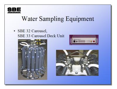
As a companion to CTD profilers, Sea-Bird supplies water sampling equipment. Sea-Bird manufactures the framework, mechanism for closing bottles, and deck power supply and sampler control. The water sample bottles for the SBE 32 are not manufactured by Sea-Bird. The SBE 32 is the portion of the equipment that triggers the bottle closure.
