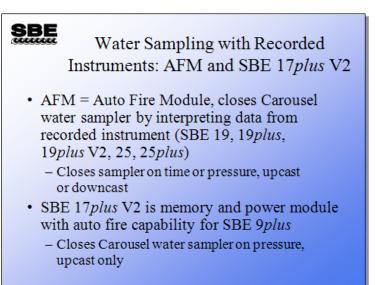
Internally recording instruments output a real-time, RS-232 serial data stream. This data stream is suitable for real-time telemetry over short cables only. The data stream is used by the AFM to monitor the depth of the sampling package for the purpose of closing water samplers.
