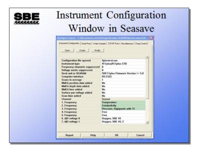
Click the Configure Inputs menu to get the Configure Inputs dialog box; the first tab is the Instrument Configuration tab. From the Instrument Configuration tab, you can open and examine an existing .con or .xmlcon file, or create a new .con or .xmlcon file.
