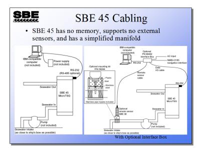
As mentioned previously, the SBE 45 does not have the capability to directly integrate remote temperature or navigational data. However, it can be used with an optional Interface Box, which accepts remote temperature and navigational data, and appends the data to the SBE 45's data stream.
