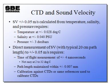
Sound velocity (SV) sensors measure the flight time of a pulse of sound between transducers. To meet the  $\pm$  0.05 m/s specification of a typical 20 cm path SV sensor, the time of flight must be measured to within about 4 nanoseconds. The electronics to perform this are difficult but feasible; however, the time delays associated with the acoustic transducers cannot be maintained over pressure and temperature.
