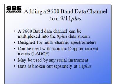
As optional equipment, a 9600-baud serial channel can be multiplexed into the 9*plus* data stream, allowing external instruments that transmit serial data at 9600 baud or less to send their data up the sea cable. This data channel was designed for multi-channel spectrometers; however, it has also been used with acoustic Doppler current meters.
