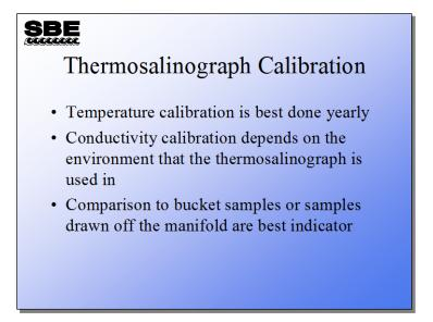
These are recommendations only; the conductivity calibration depends on the environment that the thermosalinograph is operated in.
