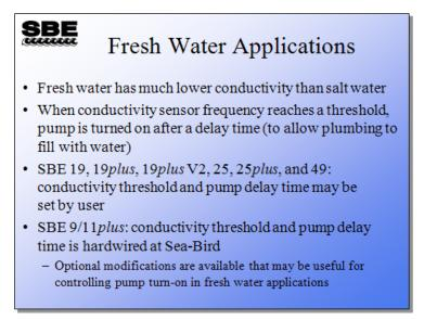
Using a CTD in fresh water requires some modification of the instrument setup for internally recording instruments or of hardware for the 9*plus*. The issue is the pump turnon signal. As delivered, Sea-Bird instruments are configured for use in saltwater. They sense the rising conductivity frequency associated with immersion in saltwater, and turn on the pump after a short delay that allows the air in the plumbing to escape.
