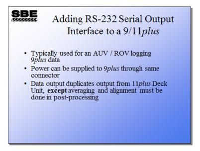
As an option, an RS-232 Serial Output interface can be installed in the *9plus*, in place of the interface for the G.O. 1015 Rosette. The *9plus* transmits the serial data through the 3-pin JT4 connector on the top end cap, at 19200 baud, 8 data bits, no parity.
