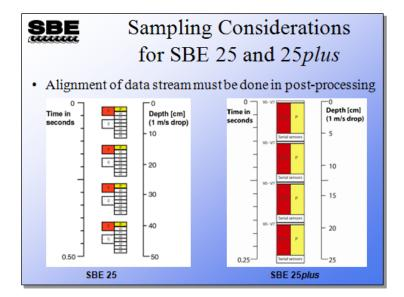
The SBE 25 has a different sampling order. Alignment of T and C must be done in postprocessing, regardless of whether the SBE 25 is used for internal recording or as a realtime instrument with a deck unit. As an internally recording instrument, the SBE 25 has the capability of averaging samples to increase the memory endurance. Averaging degrades the resolution and makes the alignment of T and C less effective.
