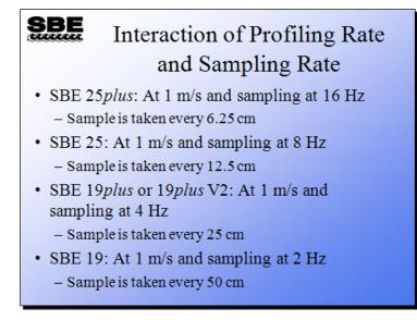
As discussed earlier, the lower sample rates of the SBE 19, 19*plus*, 19*plus* V2, 25, and 25*plus* translates into a coarser resolution than that calculated in the SBE 9*plus* example. The following page illustrates the impact that sample rate has on resolution.
