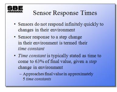
Sensors do not react infinitely quickly to a new environmental condition. For example, let's look at a 2-box ocean, with the top box at 20 °C and the bottom box at 0 °C. If our CTD moved from the top to bottom box, we would see a temperature signal that changed very quickly from 20 °C to 0 °C, but not as a perfectly sharp jump. *The reason for a slower response time for sensors is often found in the packaging of the active element of the sensor.*
