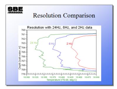
The left-most plot is data collected at 24 Hz with a nominal 1 meter/second lowering speed. The middle plot is the same data set decimated to 8 Hz to represent the resolution of the SBE 25. The right-most plot is the 24 Hz data set decimated to 2 Hz, which is representative of the resolution that would be seen with an SBE 19. The obvious conclusion is that a faster sampling rate yields higher resolution of temperature structure in the ocean temperature profile.
