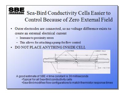
Sea-Bird's conductivity cell is a two-terminal cell, where outer electrodes are at ground and the center electrode is the signal.
