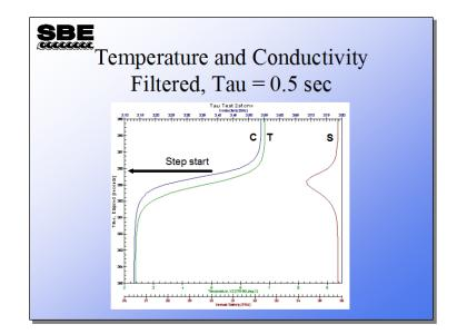
We can achieve the best salinity response by filtering the temperature and conductivity signals to give them the same time constants. It is accepted practice to filter a data channel forwards and backwards to avoid introducing a phase shift in the data. Because of this, both the leading and the trailing edge of the step response are smoothed. If only conductivity were filtered the smoothed leading edge would not match the temperature channel and a larger salinity spike would result.
