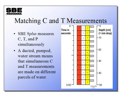
The SBE *9plus* acquisition architecture measures temperature, conductivity, and pressure simultaneously. Careful examination of the plumbing of the TC duct shows that a water parcel first encounters the SBE 3 thermistor and then transits into the conductivity cell.
