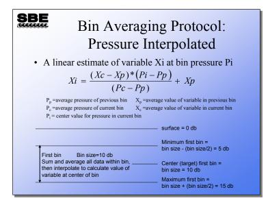
An estimate of each variable is made using the average value of that variable and pressure in the previous bin, and the average values of the variable and pressure in the current bin. Bin averaging with interpolation provides output data at regular intervals (for example, 10 meters, 20 meters, etc.).
