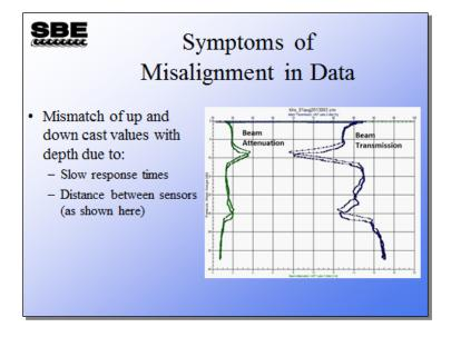
Here is data from auxiliary sensors showing misalignment.
