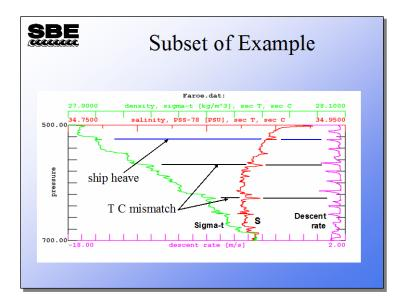
It is important to plot descent rate as well as density and salinity, because ship heave can cause errors in your data set that are completely different from alignment errors. To align your data, plot a small subset of the data that has sharp changes in temperature and/or conductivity. Look for spikes in the salinity and density that do not correspond to rapid descent rate decreases, which are indicative of ship heave.
