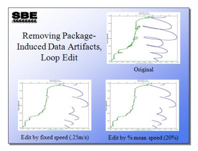
Here is the example of loopy data that we showed earlier. The bottom two plots have been edited by the two means available. Both plots show very similar results. The bottom left plot is made by editing out data that drop below a fixed speed, in this case 0.25m/s. The bottom right plot is made by editing data that drops below 20% of the mean speed calculated over a 5-minute (300-second) window; this method gives you a bit more flexibility.
