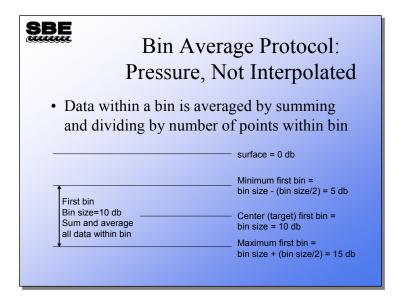
This protocol averages all the data within the bin, producing uneven bin pressures or depths. For example, if you are binning on 10-meter intervals, the first bin start is 5 meters and the end is 15 meters. All data within this window is averaged, producing a bin depth of approximately 10 meters (e.g., 10.123 meters).
