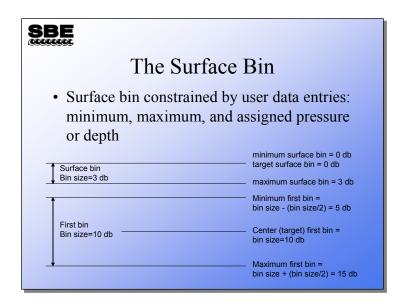
The surface bin is handled differently because the previous bin would be up in the air. The surface bin is assigned a beginning pressure or depth, an ending pressure or depth, and a target pressure or depth.
