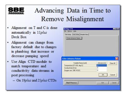
Because the 911*plus* system is well characterized, an alignment of the data stream is done automatically in the 11*plus* before data is transmitted to your computer. With the TC duct in place, an alignment of 1.75 data scans (or 0.073 seconds) is done on incoming data. A linear interpolation between scans is done to implement the alignment of a non-integer number of scans.
