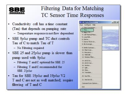
It is very desirable to match the time constants of the temperature and conductivity sensors. This improves salinity data in conditions of sharp gradients. The conductivity sensor has a time constant that depends on pumping rate; it can range from 10 millisec at a fast pumping rate to very large if no water is moving through the cell.
