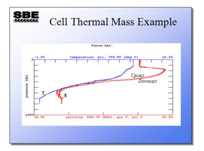
The data shown in this plot has already been aligned (using Align CTD), reducing salinity spikes associated with misalignment. We see what appears to be salinity hysteresis, but there is no temperature hysteresis. The feature that looks like salinity hysteresis is actually caused by the effect of cell thermal mass. Another way to check for cell thermal mass errors is to create a T vs S plot; the feature to look for in that plot is an open curve.
