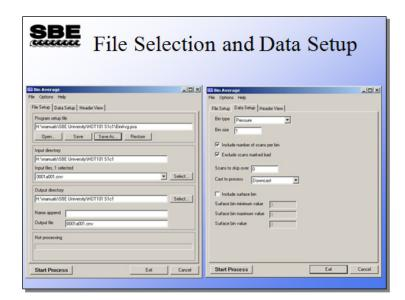
The Data Setup tab allows your choice of pressure, depth, time, or scan bins. You can include the number of scans per bin in the output file, which is useful for evaluating data from instruments with a low sample rate. Bins with 1 sample in them are not very accurate statistically.
