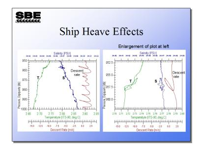
These two plots show the effect of ship heave. Both plots show descent rate in brown. The plot on the left shows that each time the descent rate drops, the temperature and salinity traces are disturbed. The plot on the right is an enlargement of a portion of the left plot, showing the loop trajectory that was mentioned previously.
