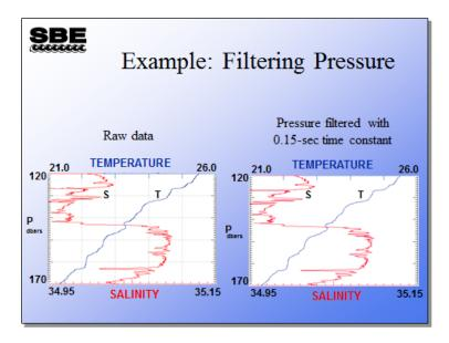
The left plot shows some *dithering* in the data that is eliminated by filtering the pressure.
