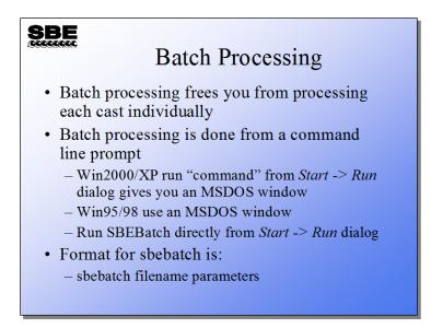
For processing large sets of cast data, batch mode processing automates the job. You can use the windows scripting host or a program provided with SBE Data Processing, SBEBatch.exe. Your batch file can take advantage of command line parameters and wild card characters.
