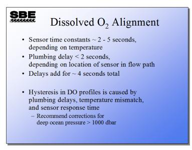
Aligning oxygen current and temperature in relation to pressure can improve hysteresis (mismatch) in dissolved oxygen profiles. The SBE 43 has a faster time constant and shows improvement in hysteresis over the Beckman- or YSI-type of sensor. Deep-ocean hysteresis corrections are advised at depths greater than 1000 dbar.
