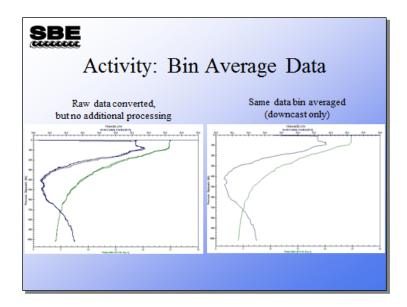
The plot on the left is one we looked at in Module 3, for data that had been converted using Data Conversion, but not yet *processed* using the advanced processing techniques we reviewed today. That plot shows both the upcast and downcast.
