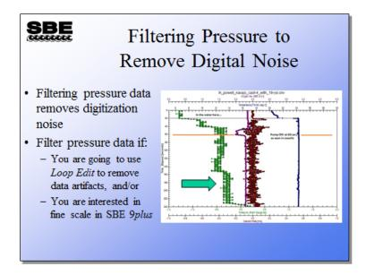
In measuring the pressure sensor signal, there is a digitization error that may be removed by filtering the signal with a low-pass filter. This has the effect of improving the resolution of the pressure signal by smoothing the digitization jitter.
