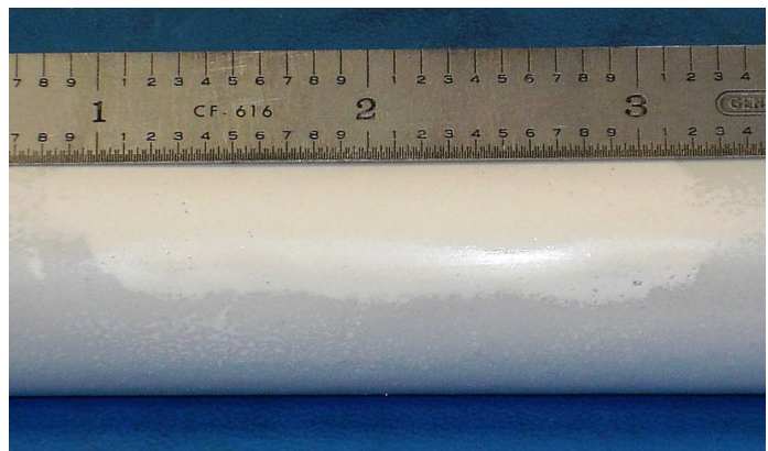
Repaired frame part. Repair has been sanded and had heat applied to restore gloss finish (steps 6A and 6B).
