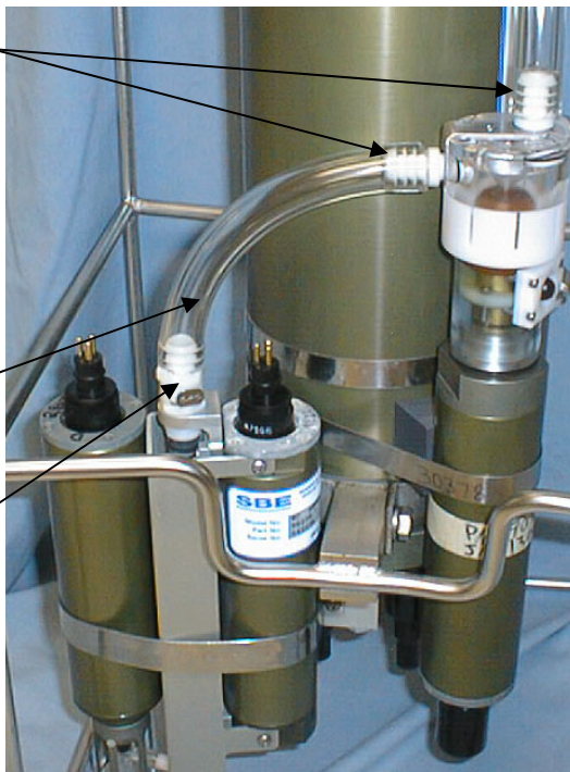
Temperature/Conductivity to DO Sensor Detail
