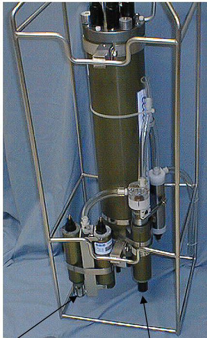
Overall View – Temperature/Conductivity Sensor Side
