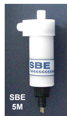
SBE 5M with plastic housing
