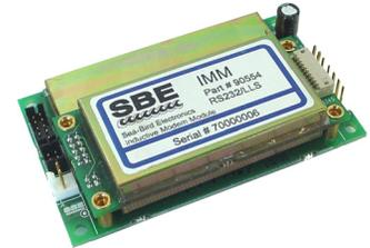
Figure 21: IMM with High Voltage Input Adapter Board
