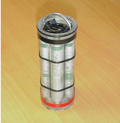
Retrofit MicroCAT battery holder
