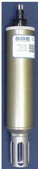
The **SBE 3F** is an enhanced version of Sea-Bird's proven SBE 3 temperature sensor. The superior performance of the SBE 3F results from its optimized electronic design combined with an extraordinarily precise calibration procedure and quality testing program. The SBE 3F has a time response of approximately 0.07 second, an initial accuracy of 0.001 °C, and is typically stable to 0.002 °C per year.
