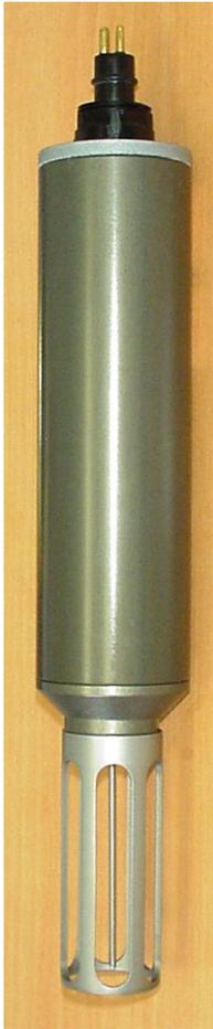
The **SBE 3S** is an enhanced version of Sea-Bird's proven SBE 3 (slow response) temperature sensor. The superior performance of the SBE 3S results from its optimized electronic design combined with an extraordinarily precise calibration procedure and quality testing program. The SBE 3S has a time response of approximately 0.6 second, an initial accuracy of 0.001 °C, and is typically stable to 0.002 °C per year.
