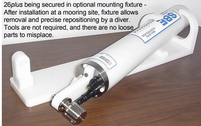
The 26plus combines Sea-Bird's non-volatile FLASH memory with a stable time base, precision thermometer, and Quartz crystal pressure sensor to provide wave and tide recording of unprecedented resolution and accuracy, along with high-quality temperature information. A second input connector for an optional SBE 4M conductivity sensor is also standard.
