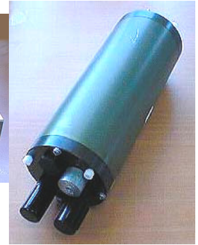
Power and Data Interface Module (PDIM)
