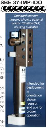
In a typical mooring, an Inductive Modem Module (IMM) or Surface Inductive Modem (SIM) housed in the buoy communicates with underwater IM instruments and is interfaced to a computer or data logger via an
