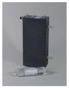
Calibration coefficients stored in EEPROM allow the MicroTSG to transmit data in engineering units.
