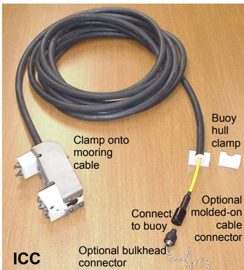
Note: ICC includes pigtail cable, conduit, and buoy hull clamp; molded-on cable connector and bulkhead connector optional.
