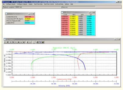
third party manufacturers (such as altimeter, fluorometer, methane sensor, nepyhelometer, PAR sensor, suspended sediment sensor, and transmissometer). What if you are using an auxiliary sensor that is not directly supported by our software? Auxiliary sensor selection includes a user polynomial, allowing you to define an equation to relate your sensor output voltage to calculated engineering units.
