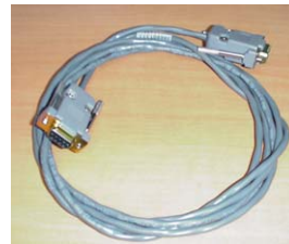
I/O cable (Interface Box to computer)
