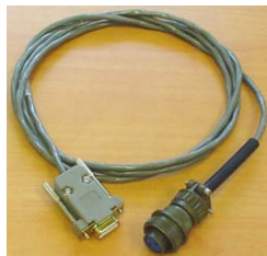
NMEA Interface test cable (Interface Box to NMEA device simulation computer)
