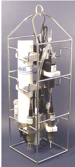
SBE 25 SEALOGGER in cage (shown with optional auxiliary sensors)
