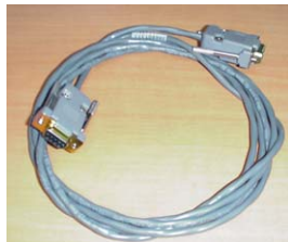
Computer to SBE 33 cable for Serial Data & Carousel Data connectors (2 cables / SBE 33)
