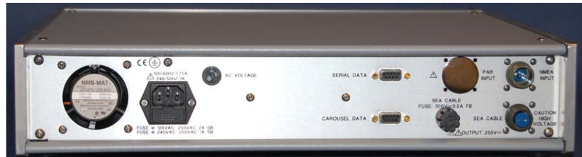
Back Panel – connectors and fuses
