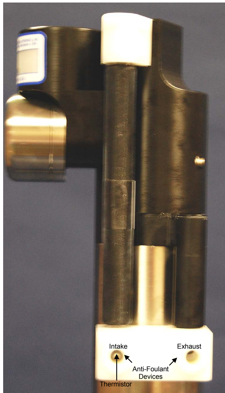
Shown with conductivity cell guard removed
