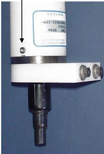
Detail - Battery/connector end cap
