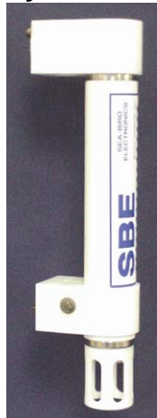
SBE 39-IM with external thermistor
