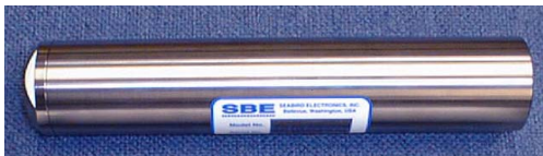
SBE 39 (with pressure) - Titanium housing, Embedded temperature sensor
