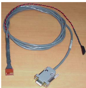
Standard I/O cable for internal I/O connector
