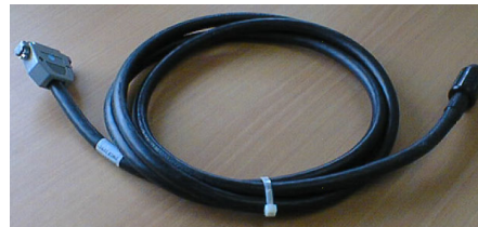
Serial Test Cable – connects UIM to computer to test serial communications through UIM's RS-232 bulkhead connector
