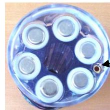
Align pin in cover plate with post hole in battery pack
