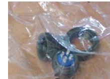
4-pin MS connector (for Sensor I/O bulkhead connector on SBE 46)
