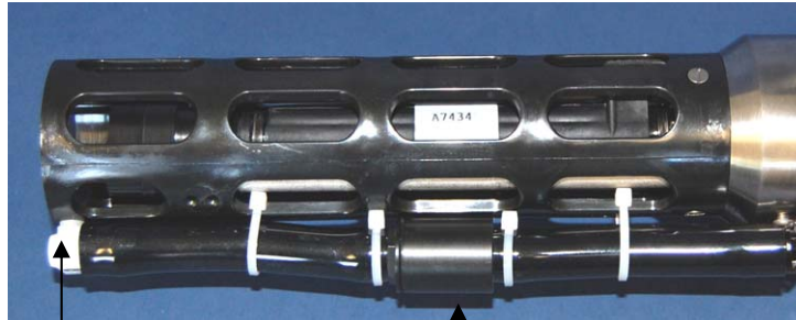
Straight exhaust shown; anti-foulant device fitting detail also applies to FastCAT with Tee exhaust.
