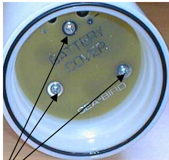
Remove Phillips-head screws and washers
