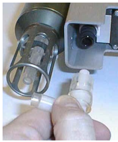
Pull C Duct straight out from conductivity cell
