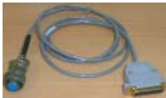
NMEA interface test cable (Interface Box to NMEA navigation device simulation computer)
