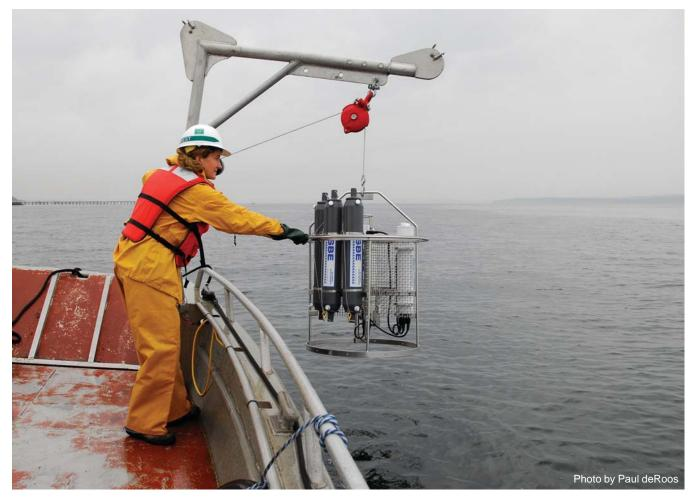
Sea-Bird's SBE 55 ECO Water sampler is a new easy-to-handle sampler with oceanographic research-quality features and small-boat compatibility. It integrates with a Sea-Bird CTD to provide autonomous water sampling at user-selected depths. The ECO Sampler's magnetically actuated lanyard release latch is derived from the SBE 32 Carousel Water Sampler and has a proven history of reliability and ease-of-use.
