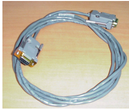
171890 9600 Baud Uplink cable
